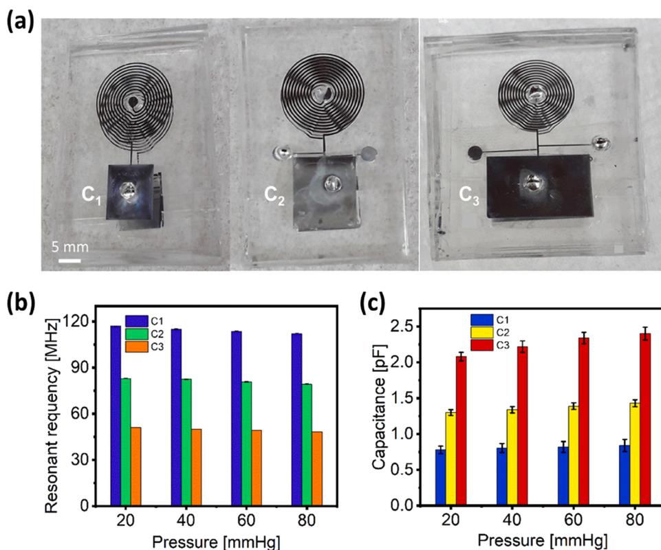
Fig. 5. Characterization of wireless capacitive sensor with different form factors. (a) Images of LC sensor fabricated with different sizes (40, 80, and 125 mm<sup>2</sup>). (b, c) Performance comparison of capacitive sensor with different sizes using saline dielectric medium.
