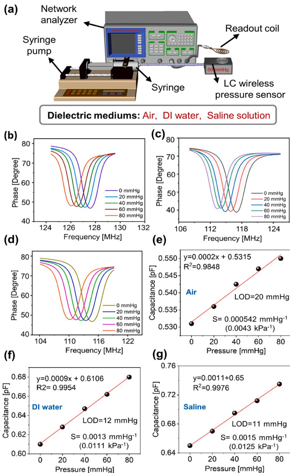
**Fig. 3.** Characterization of wireless capacitive sensor with different dielectric media under external pressure (0–80 mmHg). (a) Experimental setup used to study the performance of capacitive sensor. Influence of pressure on resonant frequency of the sensor with (b) air, (c) DI water, and (d) saline solutions (e, f, g) capacitance of the pressure sensor with different dielectric mediums.
