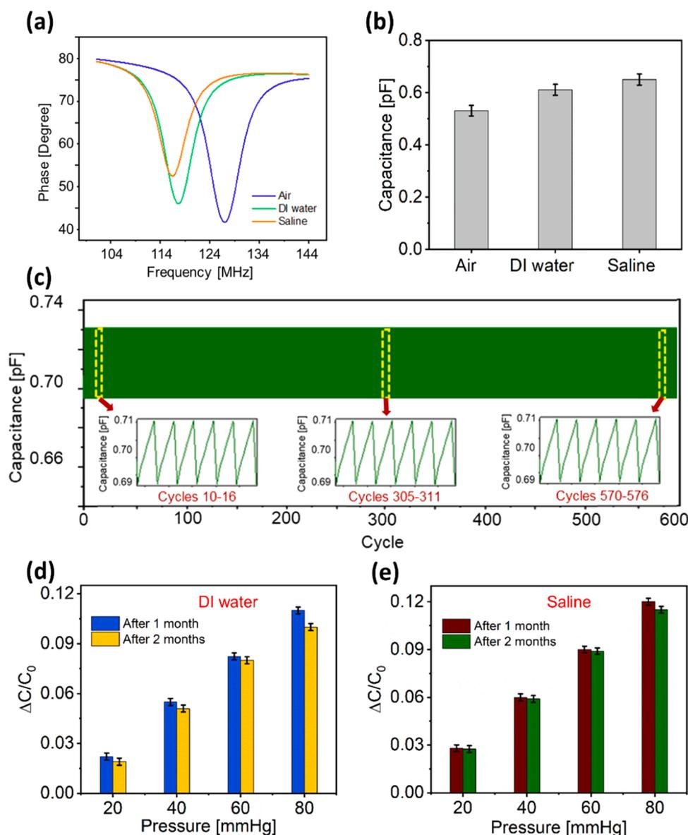
**Fig. 4.** Comparison of capacitive sensor performance with different dielectric media: (a, b) air, DI water, and saline solution. Durability and robustness study of wireless capacitive sensor, for (c) loading and unloading of 600 cycles, (d) two months with DI water as dielectric layer and (e) two months with saline as dielectric layer.
